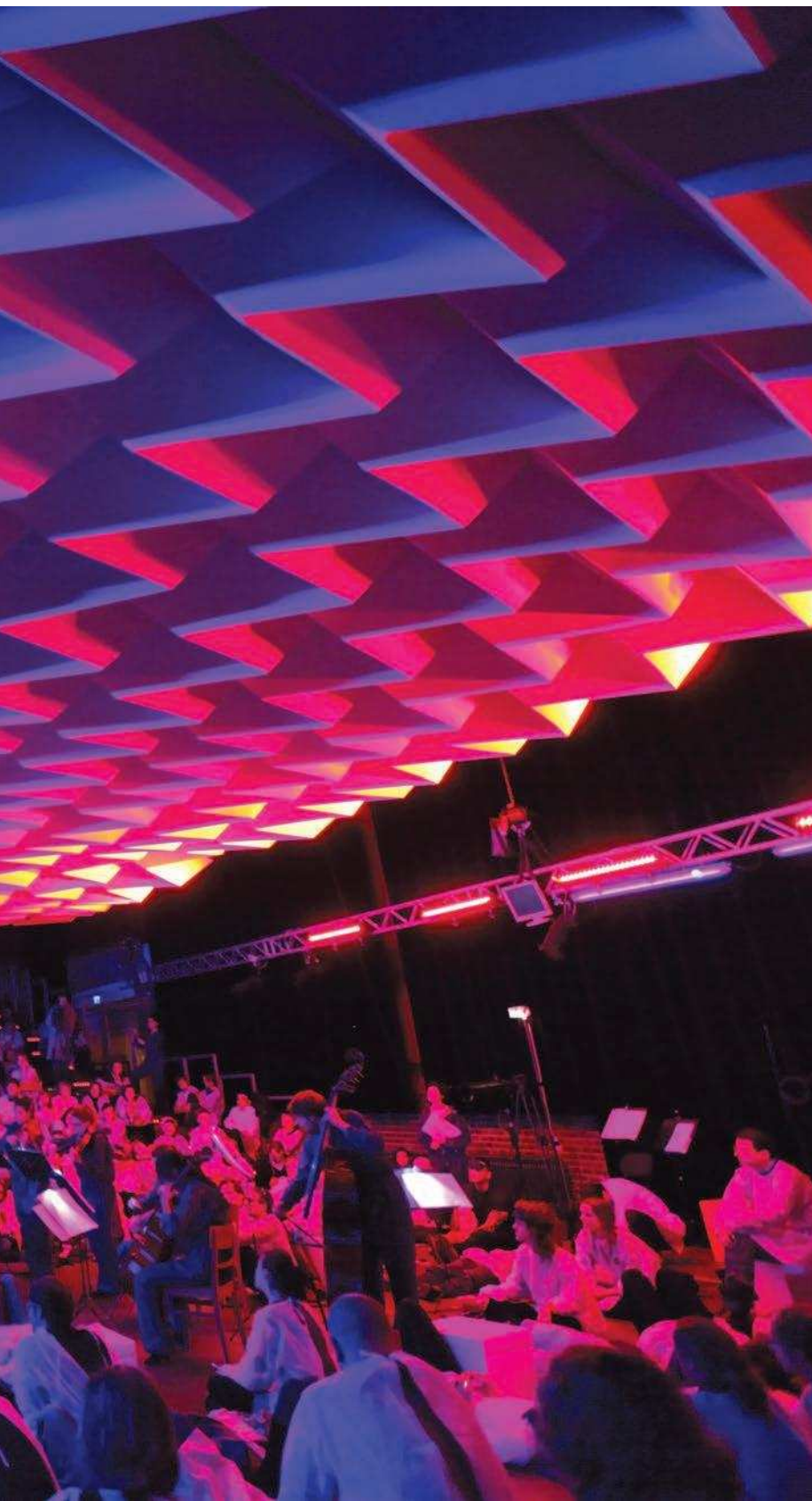
This huge multi-V-grid ceiling was made from hundreds of parallelograms of corrugated cardboard and suspended above a concert-going audience. A complex manually-operated lever system above it enabled different sections of the ceiling to rise and fall dramatically like a swelling sea, in reaction to the music. Dimensions: 25m x 11m (81ft x 36ft). Designed by Anna Kubelik (Germany).
